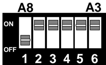
Figure 2 - DIP-Switch Illustration
