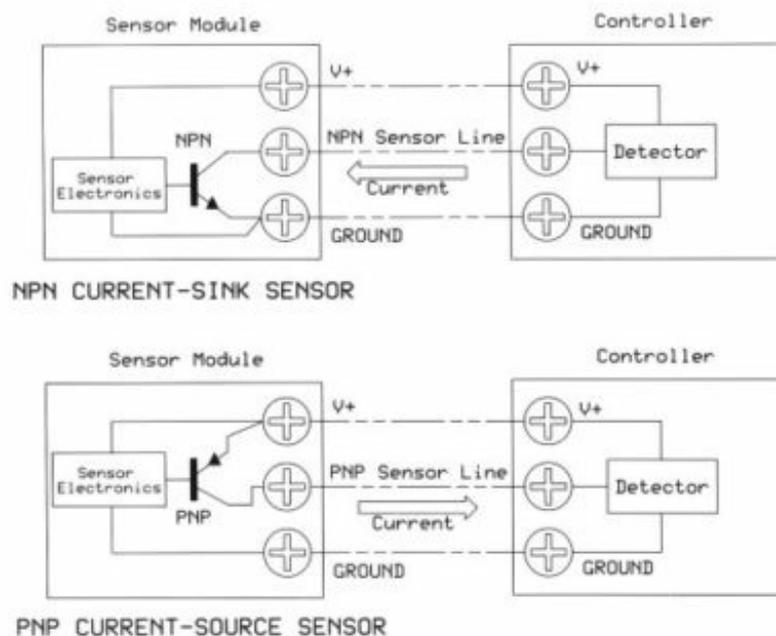
**Figure 12.** These diagrams show how current flows in an NPN and a PNP sensor connected to a compatible controller. Compare these circuits with the LED-control circuits in Figures 10 and 11.
