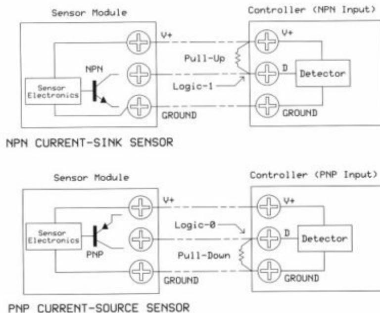
**Figure 13.** When the PNP and NPN transistors turn off (shown as disconnected here), no current flows to or from the Detector so we don't know for sure what voltage—if any—the detector input “sees.” An added pull-up or a pull-down resistor supplies the proper logic level when transistors turn off. Each input requires its own resistor.
