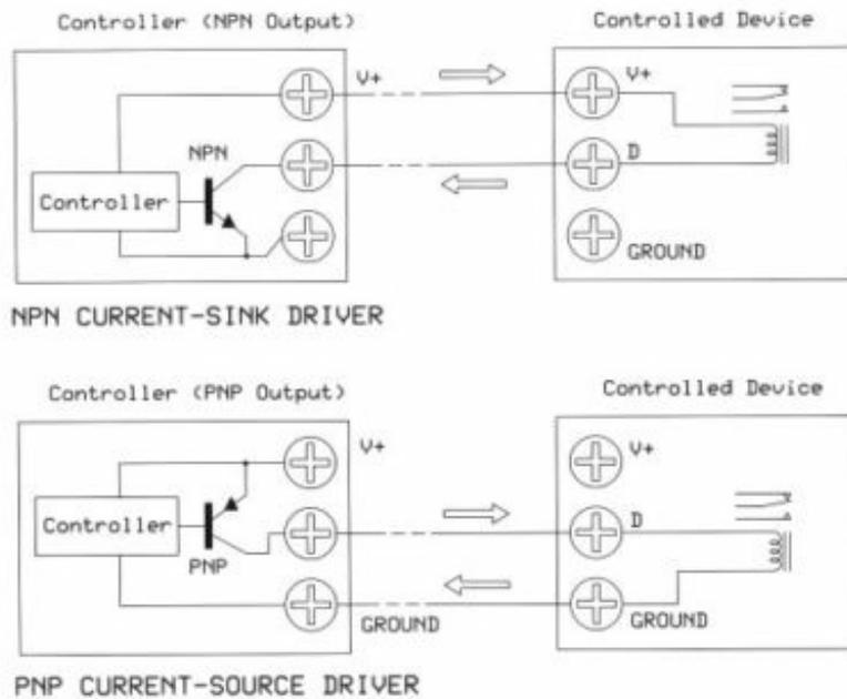
**Figure 15b.** The NPN or PNP outputs also may serve as current sinks or sources that require no pull-up resistors. Here the open-collector outputs control on-off current through a relay coil.
