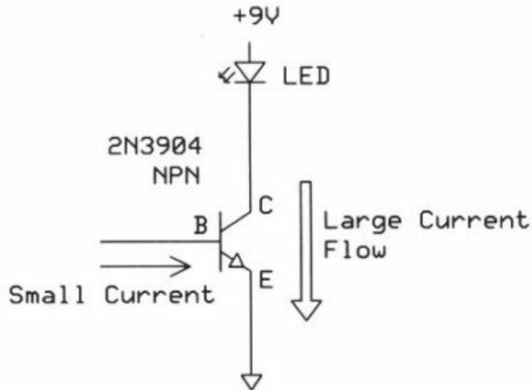
**Figure 10.** An NPN transistor controls current flow through an LED. A small current into the base turns on the transistor just a bit. A higher current into the base lets a higher current flow and the LED becomes brighter. Think of this circuit as a *current sink* because the LED connects directly to the higher potential and the transistor connects directly to ground.
