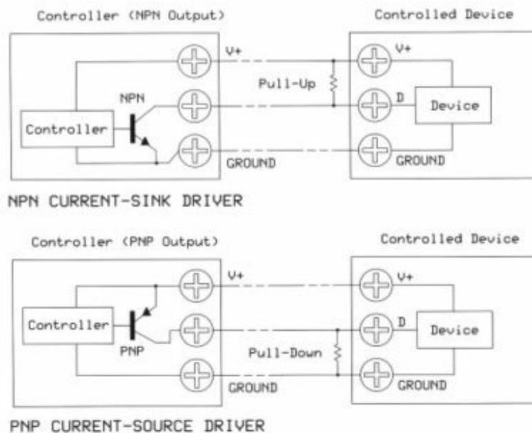
**Figure 15a.** A controller or I/O module may offer either NPN or PNP outputs. In these circuits the controller supplies a logic level of either ground or V+ to the controlled device.
