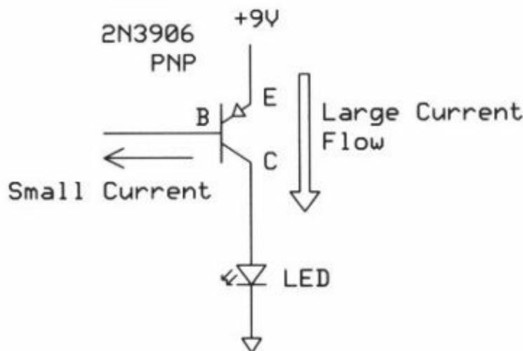
**Figure 11.** This circuit shows how current drawn from a PNP transistor base controls the flow of current from the emitter to the collector. This circuit is equivalent to a *current-source* because it controls the flow of current from the highest potential to the load that connects directly to ground.
