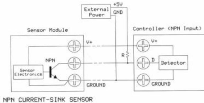
**Figure 14.** An example of a pull-up resistor and a separate 5-volt power supply used with an NPN current sink to produce logic levels independent of the power-supply voltage in the controller or the sensor. The 5-volt power-supply ground must connect to the ground between the sensor and the controller.
