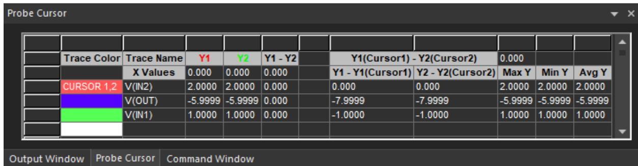
The *Probe Cursor* window shows the value of the output voltage corresponding to the values of the input voltages and resistances according to the formula of the inverting summing amplifier:
