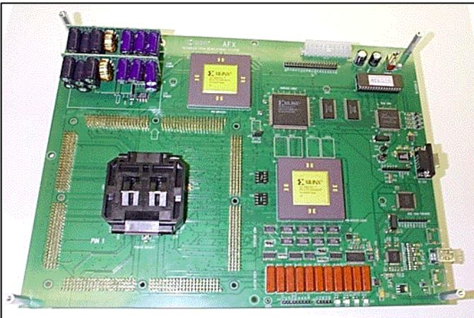
Figure 1: AFX motherboard used for SEE testing of the *Virtex* FPGA. Support circuitry interfaces to a PC and allows for
