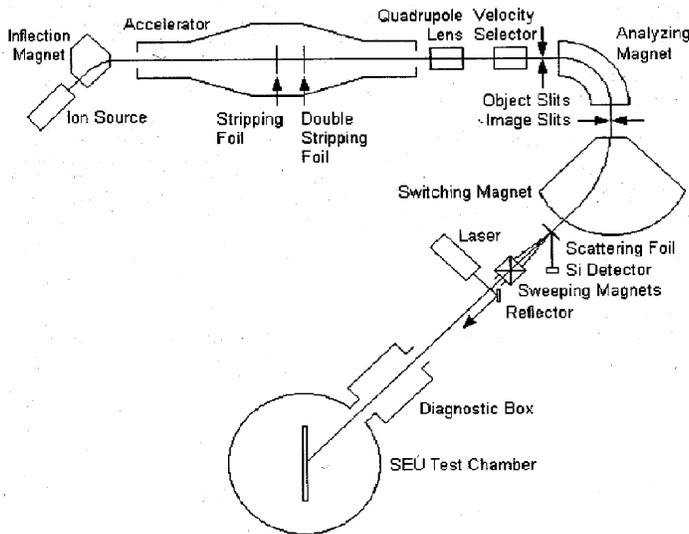
Figure 1. Layout of the beam line.
