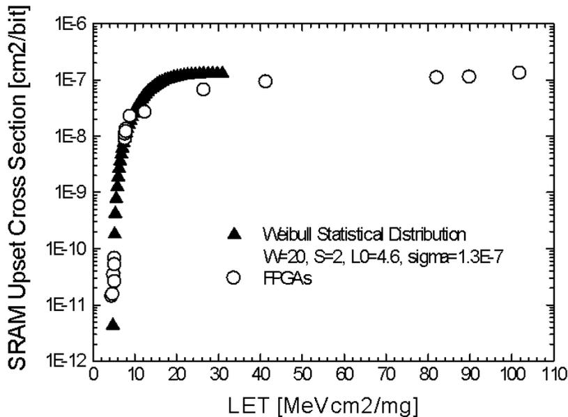
Figure 2. Xilinx XQR4036XL RAM upset cross section versus LET. The dashed curve uses the Weibull model.
