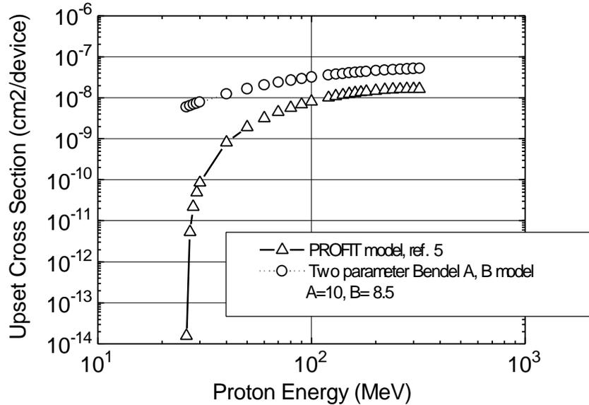
Figure 3. Predicted proton upset cross section versus proton energy from the PROFIT and the two-parameter Bendel models.
