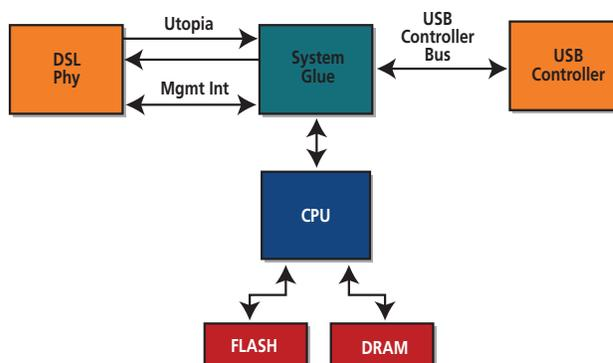
Figure 4 - DSL Modem with USB Host Interface
