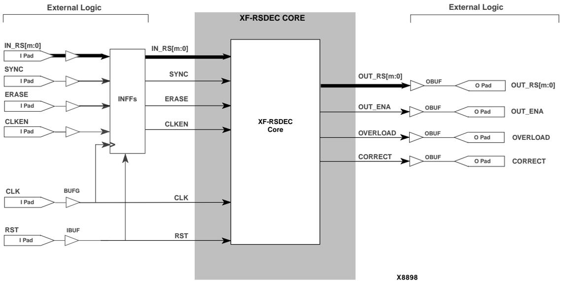
Figure 1: XF-RSDEC Core with External Logic (Examples 2 and 3)
