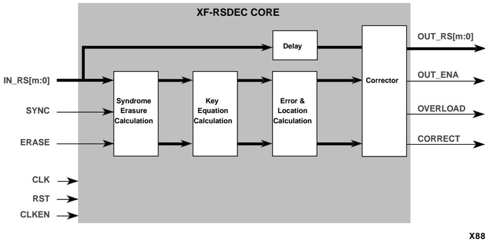
Figure 2: XF-RSDEC Core Block Diagram (Examples 2 and 3)
