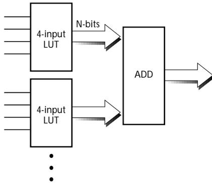
**DSP functions can be broken down into LUT / accumulate implementations that are a perfect fit with the Xilinx FPGA architecture.**
