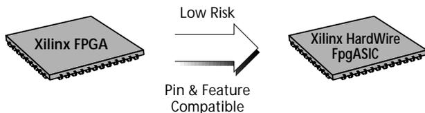
For high volume production, FPGAs can be automatically converted to an ASIC equivalent through the Xilinx patented HardWire conversion process. All of the conversion is done by Xilinx, and no new test vectors are required. You can move on to the next project instead of spending valuable time on cost reduction. This is the fastest way to the lowest cost production solution. HardWire devices can reduce the cost of a programmable solution by as much as 90%.
