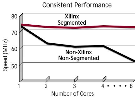
**DSP LogiCORE modules use only local routing resources. This 12-bit multiplier core benchmark illustrates the performance and predictability of Xilinx DSP over competing FPGAs.**
