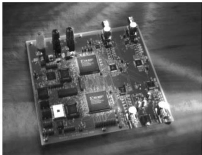
**Xilinx DSP development board contains two analog channels, two Xilinx FPGAs, and one TI 320C54 series DSP processor. Available from AllianceCORE partner.**
