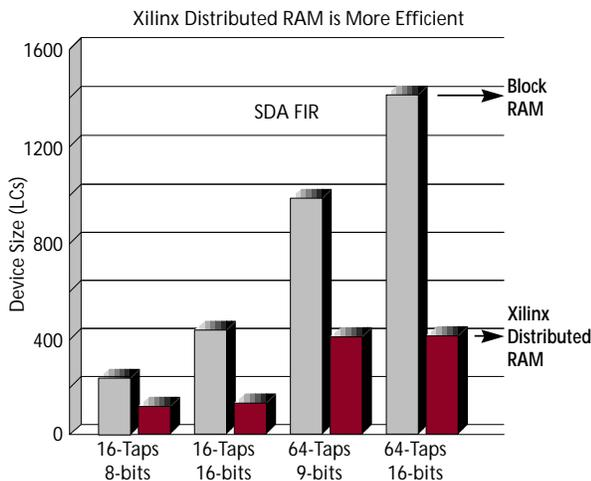
**Distributed RAM makes possible the implementation of a time-skew buffer in RAM instead of flip-flops, resulting in a 50% reduction in filter size.**
