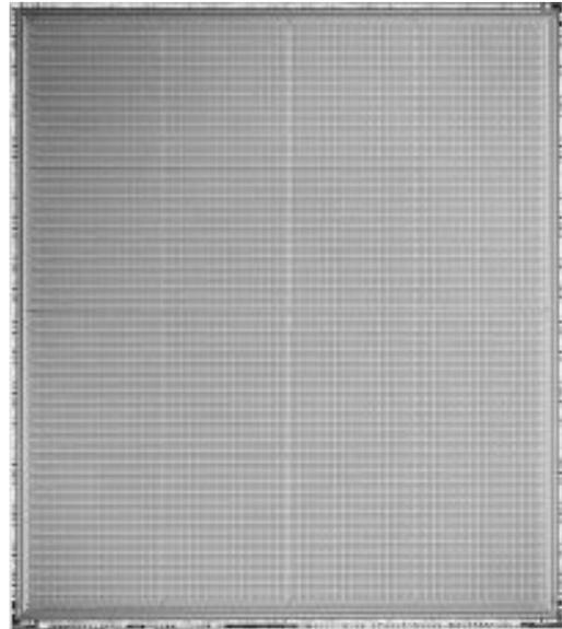
**Die Photo illustrates the regular, scalable structure of the distributed memory architecture of Xilinx FPGAs**
