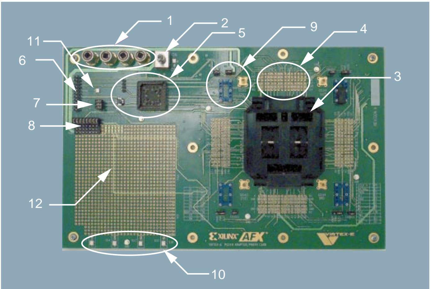
**Figure 2: Detailed Description of Xilinx Prototype Board Components**
