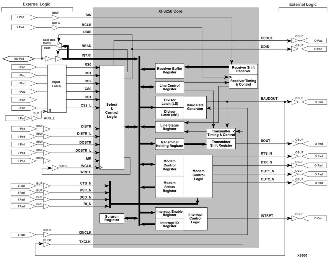
Figure 1: XF8250 Asynchronous Communications Core Block Diagram
