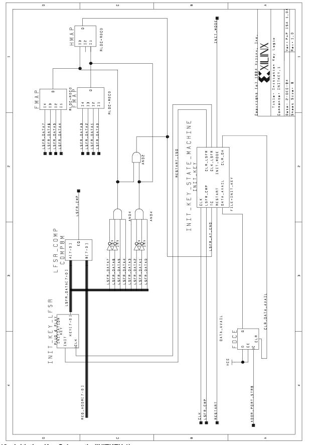
Figure 18—Initiation Key Schematic (INITKEY.1)
