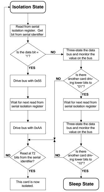
of the serial identifier which is being examined one bit at a time. The response is controlled by the isolation ABEL state machine defined in Figure 16.
