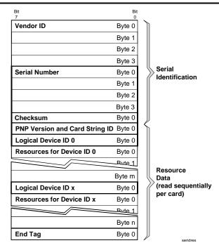
Figure 6. Serial Identifier and Resource Data
