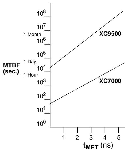
Figure 2: LOG MTBF versus t<sub>MET</sub>
