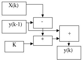
Figure 3- Pixel Calculation implementation for Kalman filtering.
