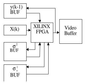
Figure 2- System level implementation for Kalman filtering.
