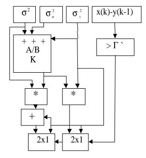
Figure 4- Parameter Calculation implementation for Kalman filtering.
