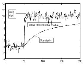
Figure 1- The result of Kalman filtering, using motion detection, in comparison with non-adaptive filtering when SNR is 20dB and  $\Gamma$ =3.29.
