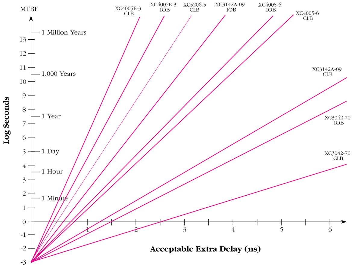
XC4005E-3 and the XC3142A-09; and, for comparison purposes, two older-technology devices, the XC4005-6 and the XC3042-70. In each device, two different implementations test the IOB and CLB flip-flops. The XC5200-5 CLB flip-flop was also tested. (There is no IOB flip-flop in XC5200 architecture.)
