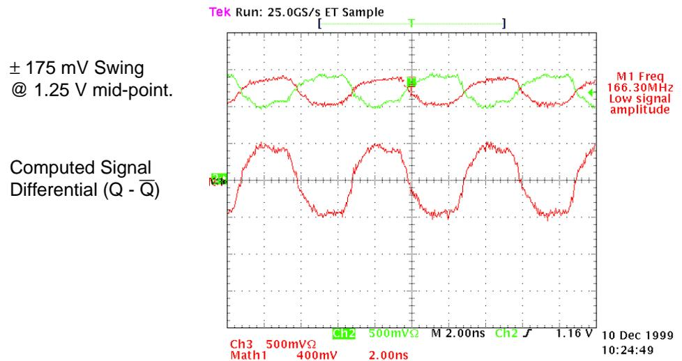
Figure 4: LVDS Output Waveform
