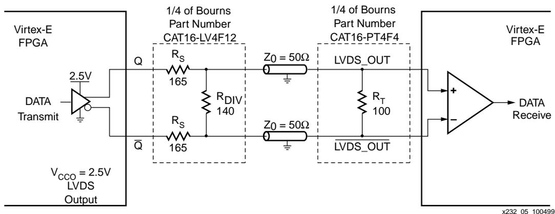
Figure 2: Virtex-E LVDS Line Driver and Receiver Schematic
