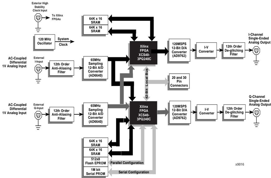
Figure 2: GVA-220 Spartan FPGA Block Diagram
