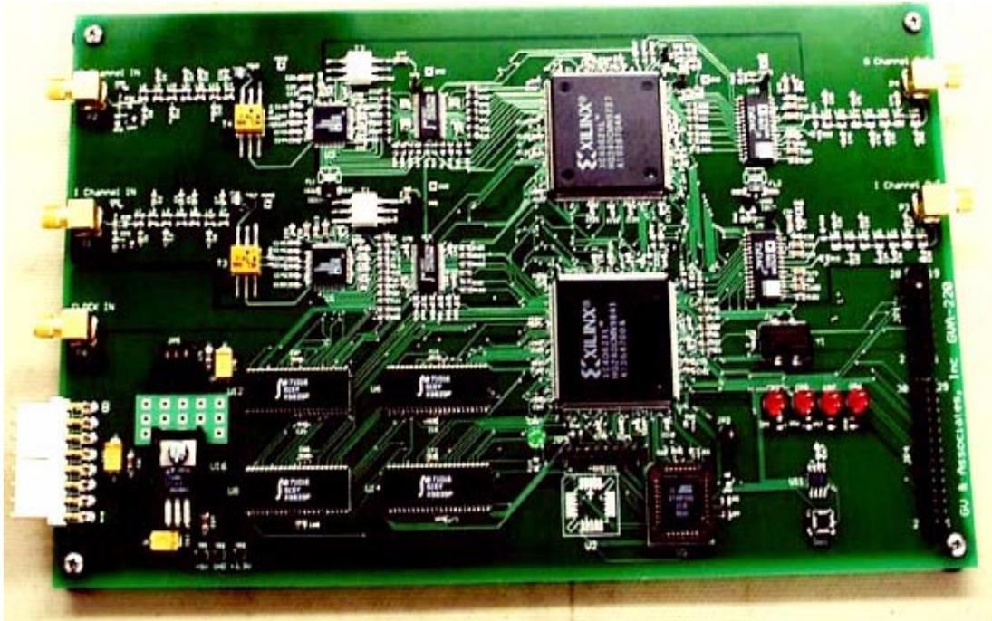
Figure 1: GVA-220 DSP Hardware Accelerator
