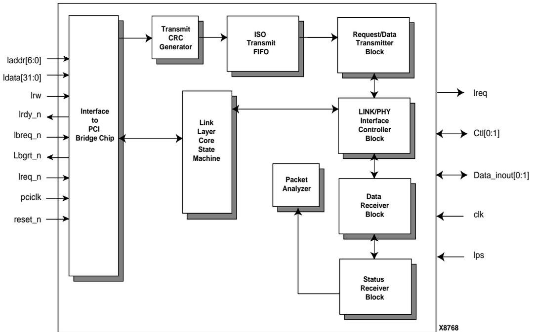
Figure 1: IEEE 1394 FireWire Link Layer Core Block Diagram
