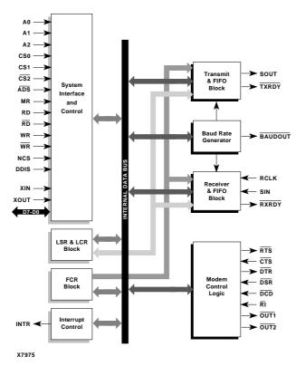
Figure 1: M16550A Block Diagram
