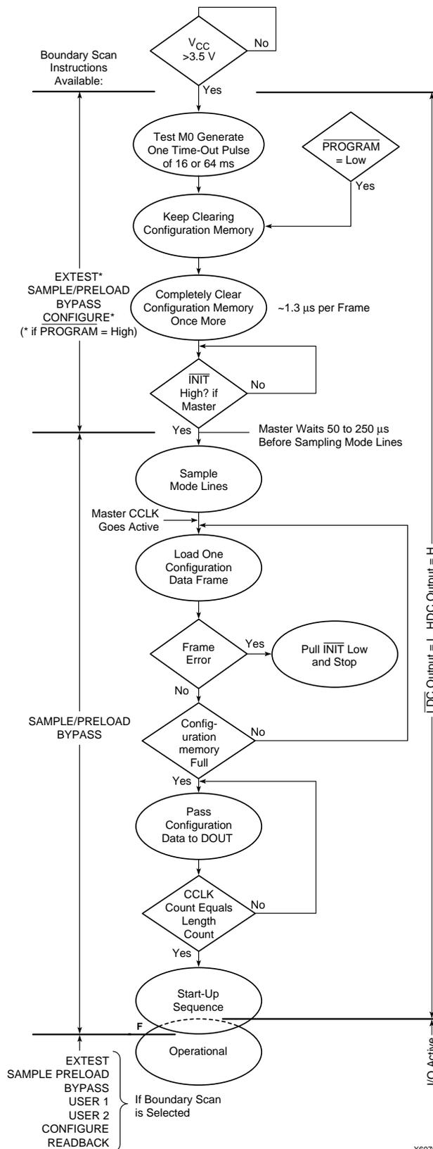
Figure 4: Power-up Configuration Sequence
