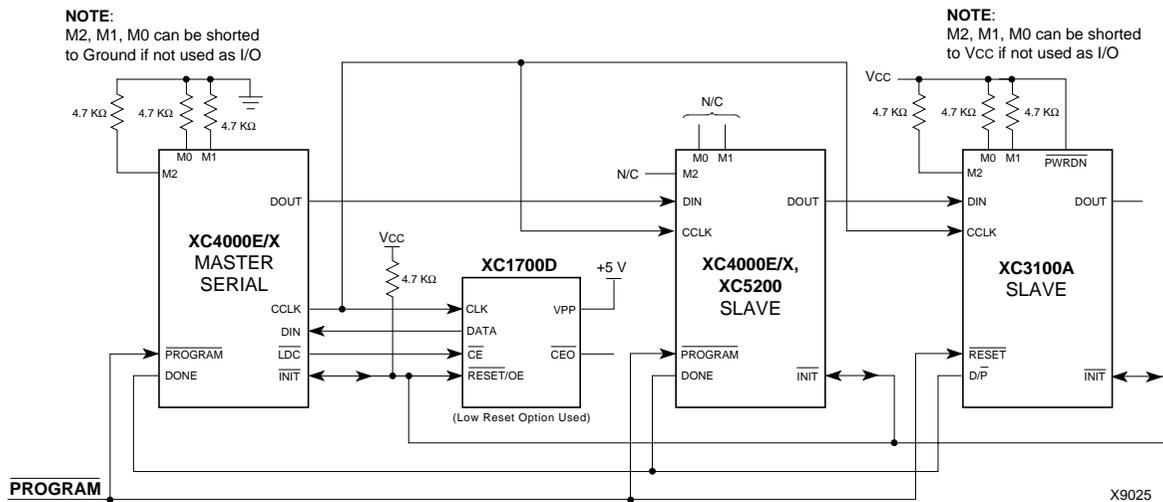
Figure 9: Master/Slave Serial Mode Circuit Diagram
