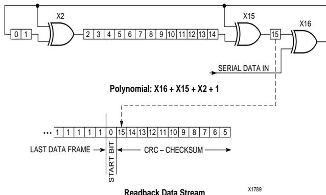
Figure 3: Circuit for Generating CRC-16
