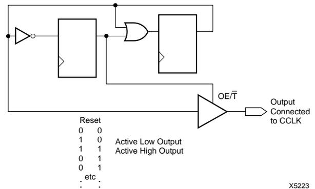
**Figure 2: CCLK Generation for XC3000 Master Driving an XC4000 Series Slave**
