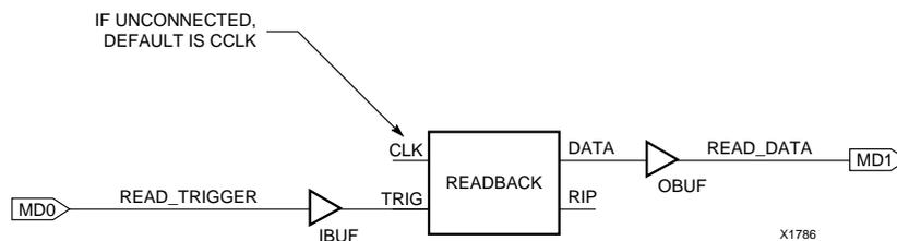
**Figure 7: Readback Schematic Example**
