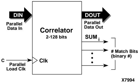
Figure 5. Core Schematic Symbol – Parallel Data In
