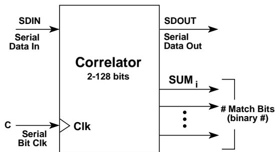
**Figure 4. Core Schematic Symbol – Serial Data In**
