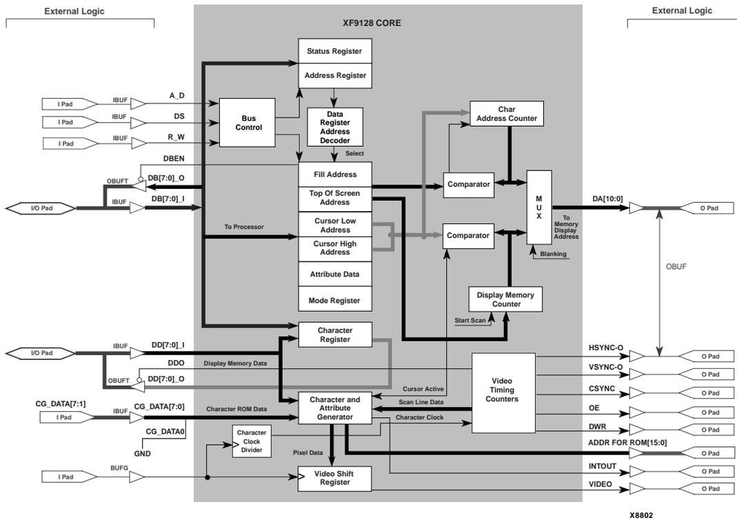
Figure 1: XF9128 Video Terminal Logic Controller Block Diagram
