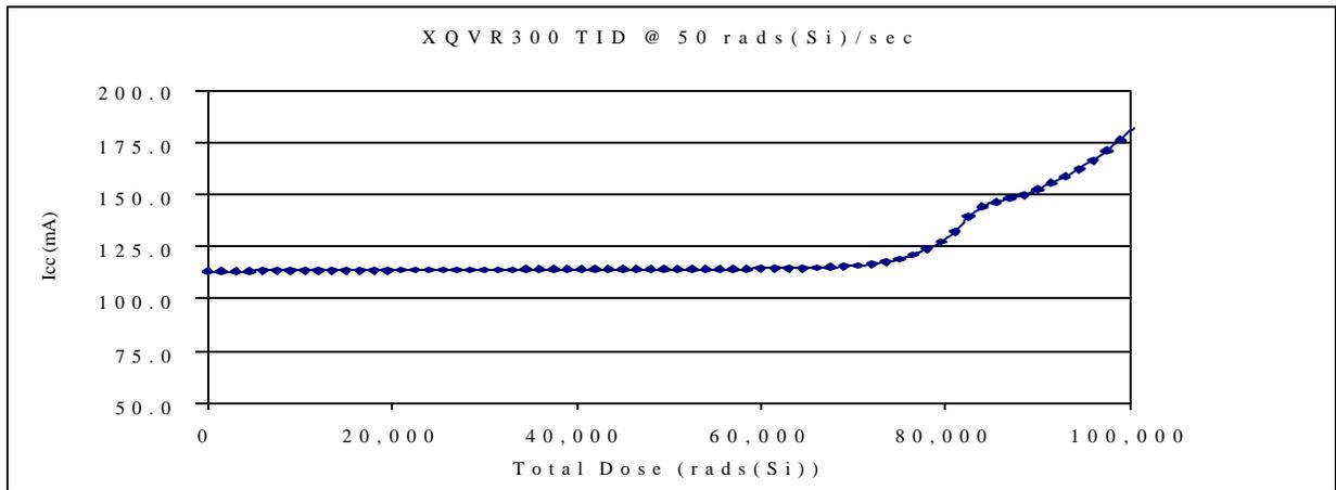
**Figure 1. A comparison of the effect of dose rate on the leakage performance of a 0.25 $\mu$ M FPGA technology utilizing Trench Isolation**
