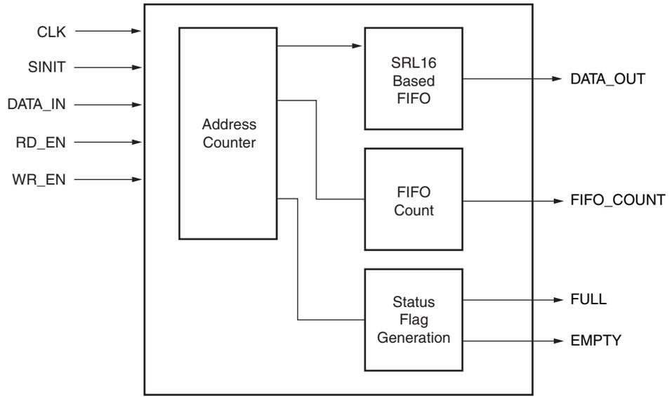
Figure 1: Synchronous FIFO Using SRLC16 Shift Registers
