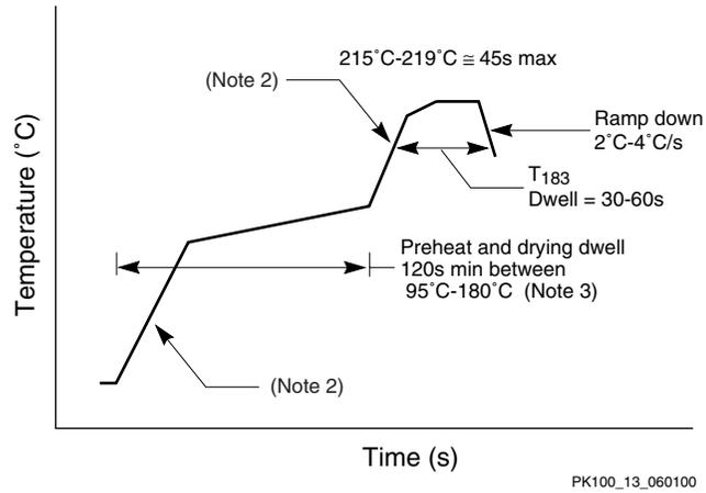
Figure 13: Typical Conditions for Vapor Phase Reflow Soldering
