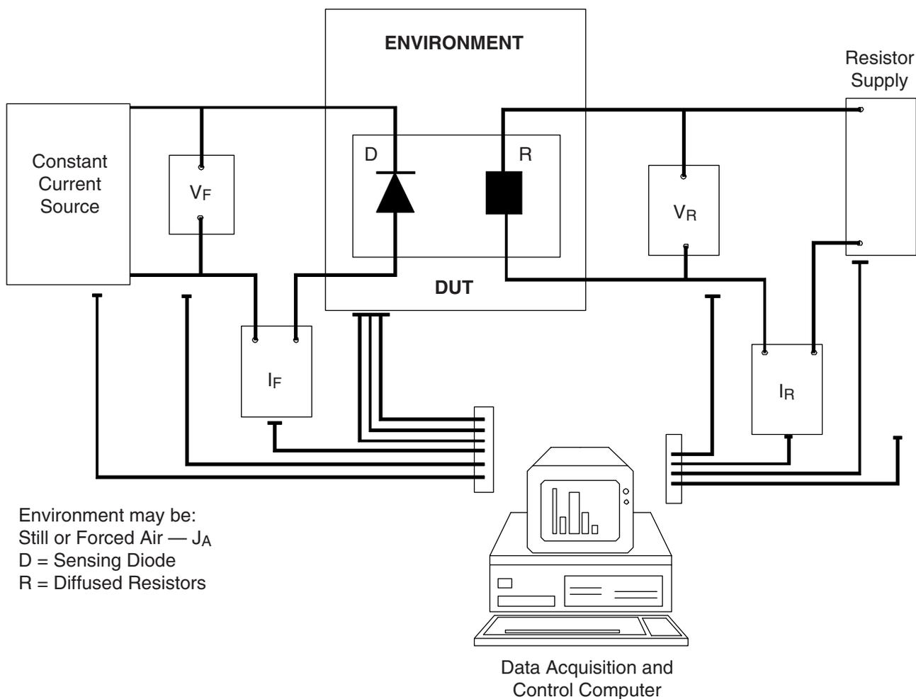
Figure 3: Thermal Measurement Set-Up (Schematic for Junction to Reference)
