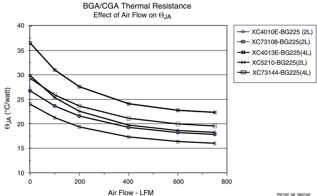
Figure 8: **BGA/CGA Thermal Data** (Effect of Air Flow on  $\theta_{JA}$ )
