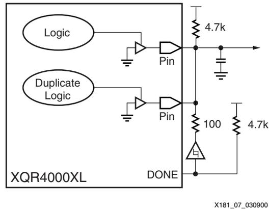
Figure 7: Wire-ANDing Critical Outputs
