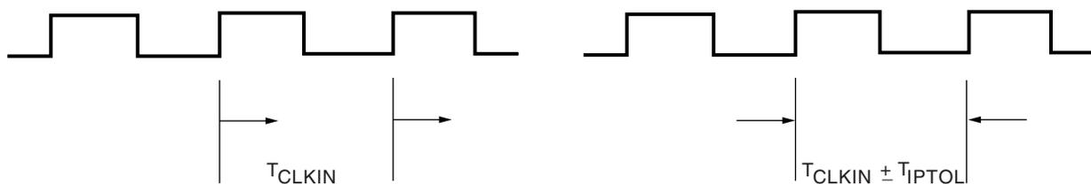
**Clock Jitter:** the difference between an ideal reference clock edge and the actual design.
