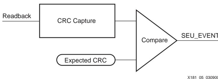
Figure 5: Readback CRCComparator
