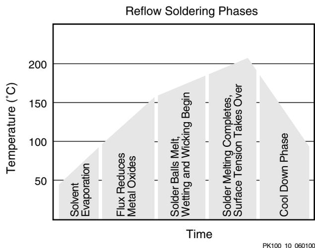
**Figure 10: Soldering Sequence**
