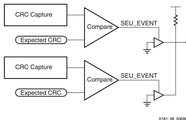
*Figure 6: Redundant CRC Comparator*
