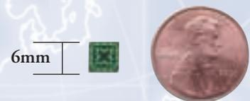
Figure 2 - Xilinx CoolRunner CPLD in a chip scale package – small, light, and ultra low power
