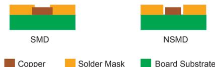
Figure 2 - Cross section of SMD and NSMD pads
