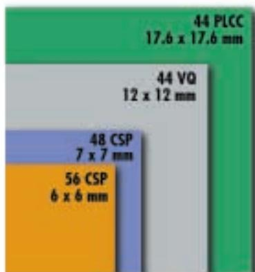
Figure 1 - A 56 CSP (CP56) occupies 11% of the space of a 44 PLCC and offers 33% more I/Os.
