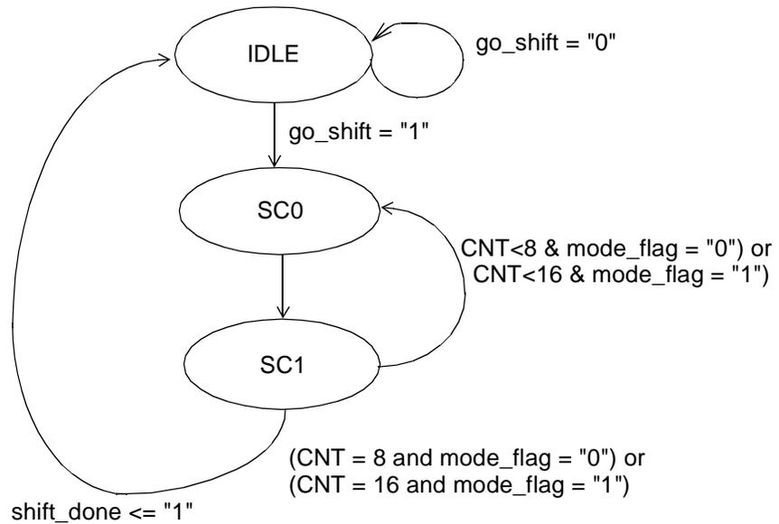
Figure 7: SHIFT State Machine Control Logic
