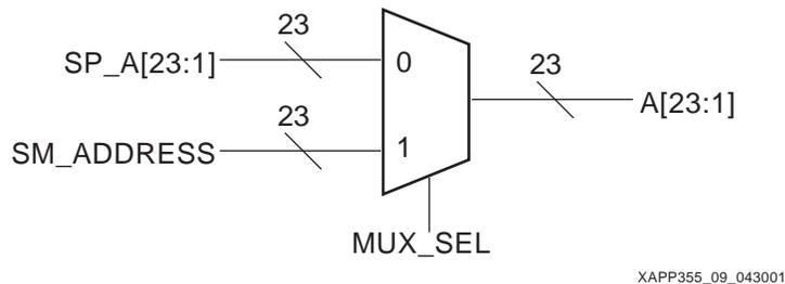
Figure 9: Address MUX
