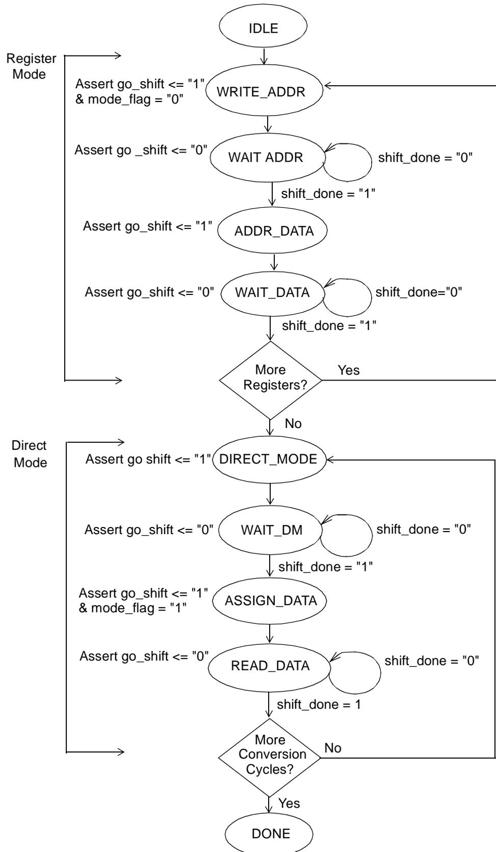
Figure 6: MAIN State Machine Control Logic
