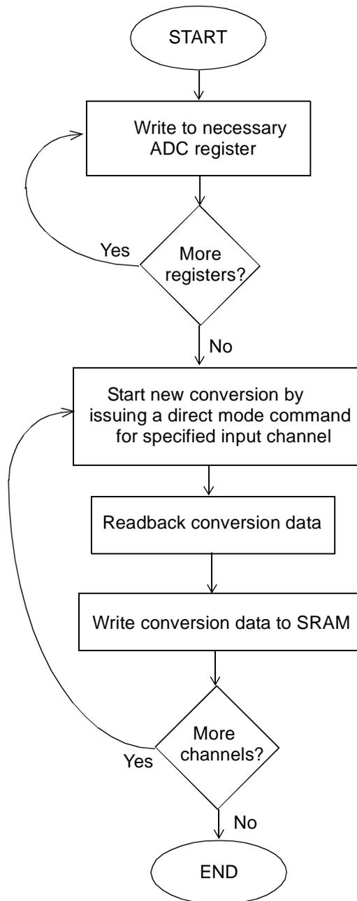
Figure 5: ADC Interface Operational Flow
