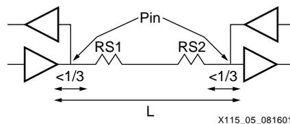
Figure 5: Bidirectional Series Termination
