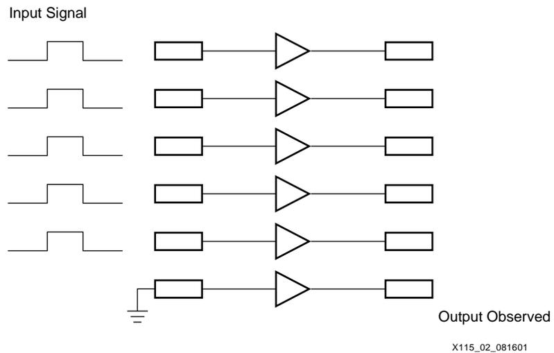
Figure 2: Ground Bounce Measurement
