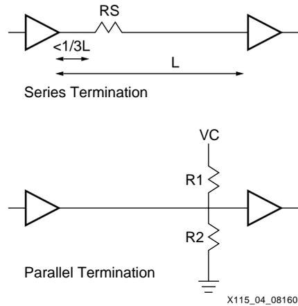
Figure 4: Single Ended Series/Parallel Termination
