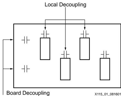
Figure 1: Board V<sub>CC</sub> Decoupling
