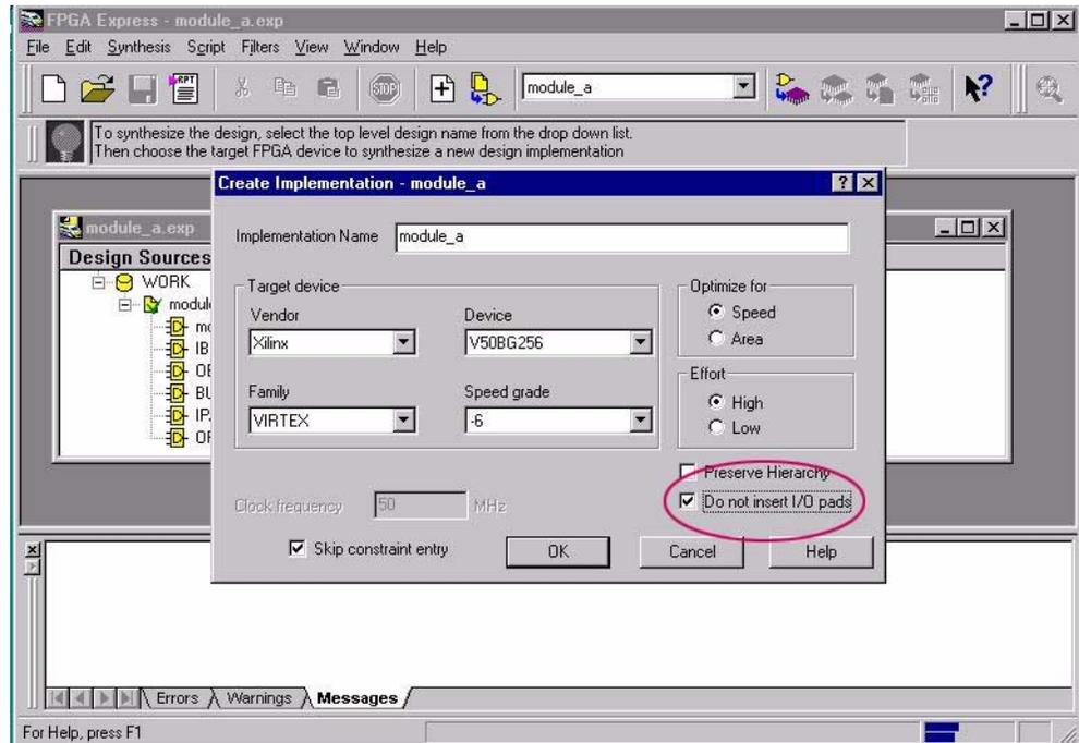
Figure 5: Disabling I/O Insertion in FPGA Express
