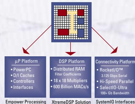
Figure 2 - A single FPGA platform for multiple applications
