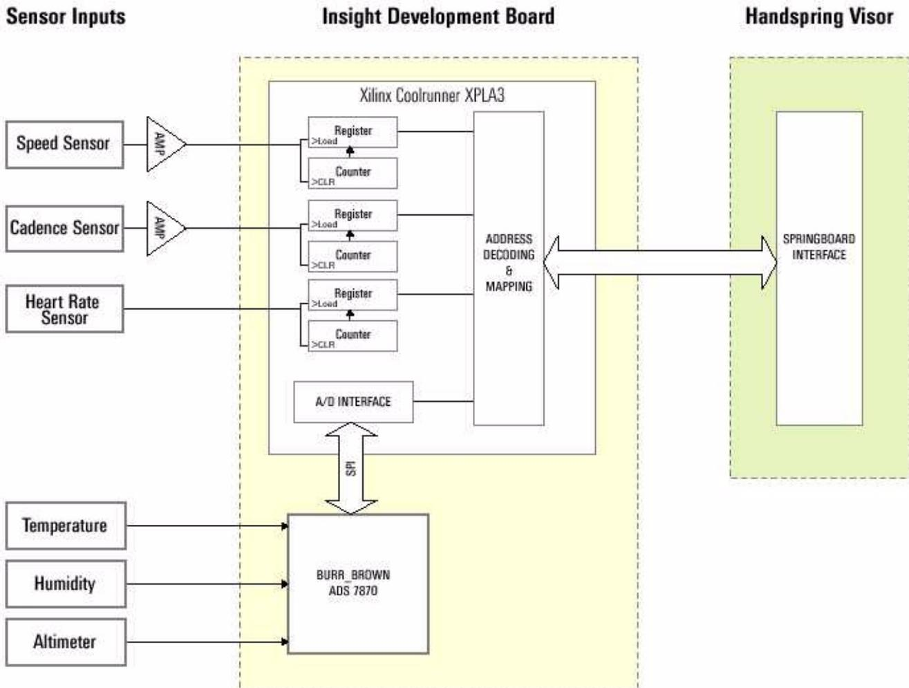
Figure 5: Cool Trak Block Diagram
