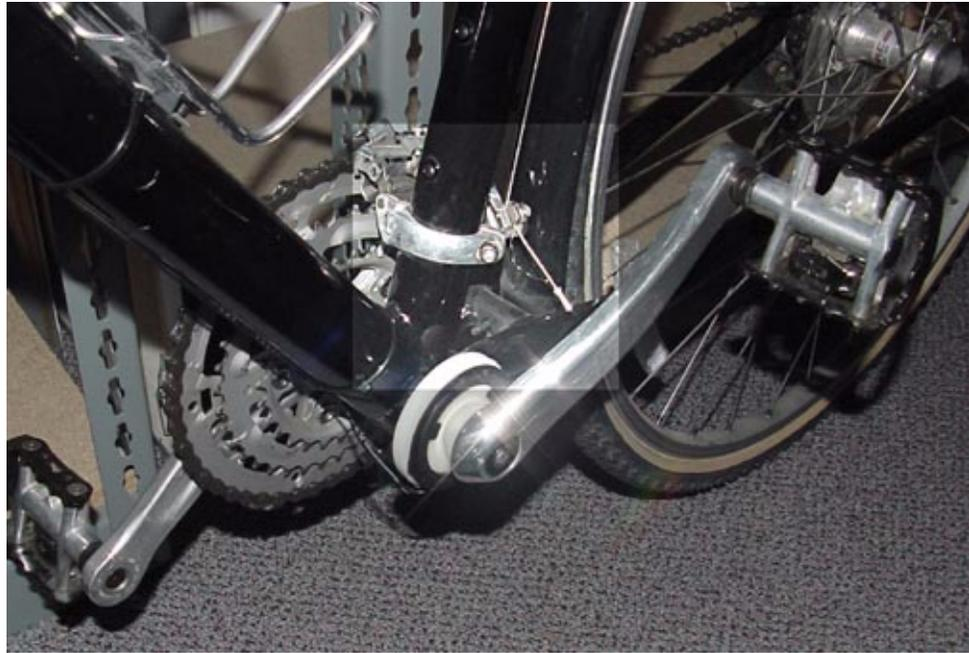
*Figure 7: Cadence Sensor Located On Bicycle Crank*
