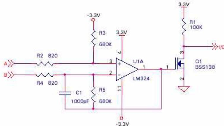
Figure 6: Differential Amplifier Circuit
