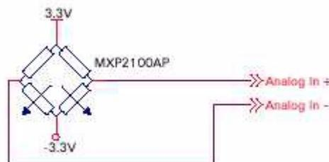
Figure 10: Altimeter/Barometer Circuit
