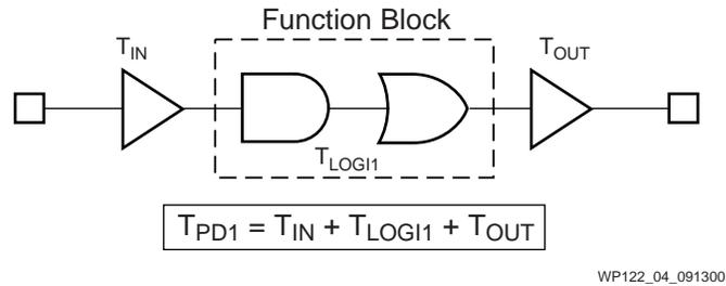
Figure 4:  $T_{PD1}$  with a Single Product Term
