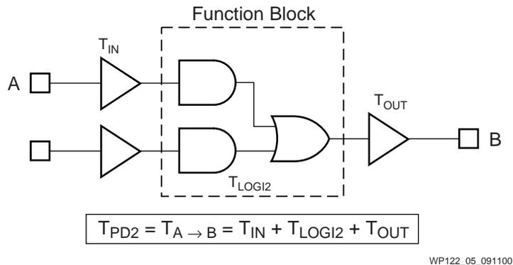
Figure 5:  $T_{PD2}$  with Two to 48 Product Terms
