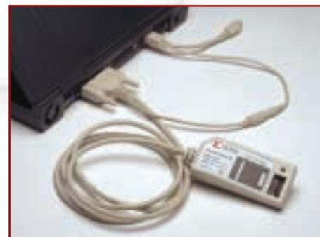
Parallel Cable IV connected to PC
