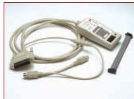
Parallel Cable IV with ribbon cable connector
