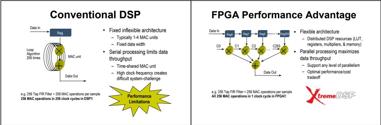
Figure 4 – Conventional DSP versus DSP Functions in FPGAs
