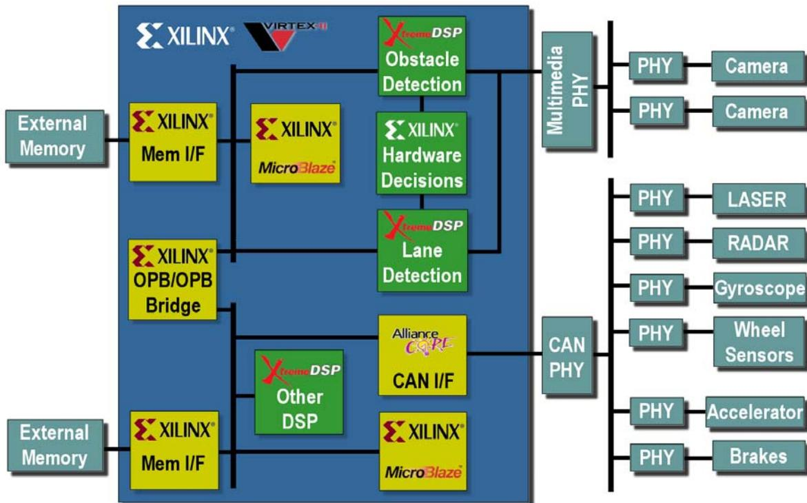
Figure 3 - Concept of FPGA in ACC Driver Assistance System
