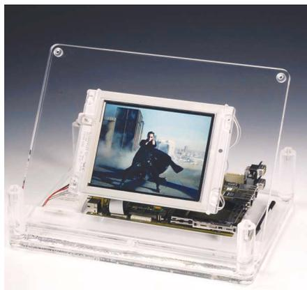
Figure 2 - Acunia automotive development platform with Xilinx Spartan-II FPGA and CoolRunner™ CPLD onboard
