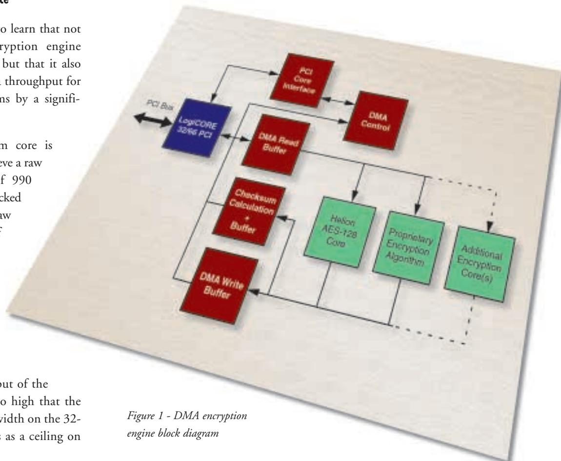
Figure 1 - DMA encryption engine block diagram
