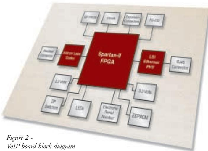
Figure 2 - VoIP board block diagram
