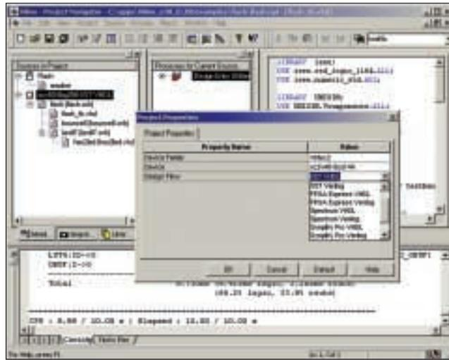
Figure 1 - Integrated synthesis options available in ISE
