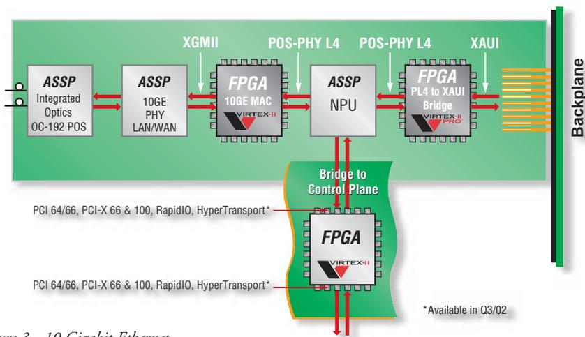
Figure 3 - 10 Gigabit Ethernet LAN/WAN line card application example
