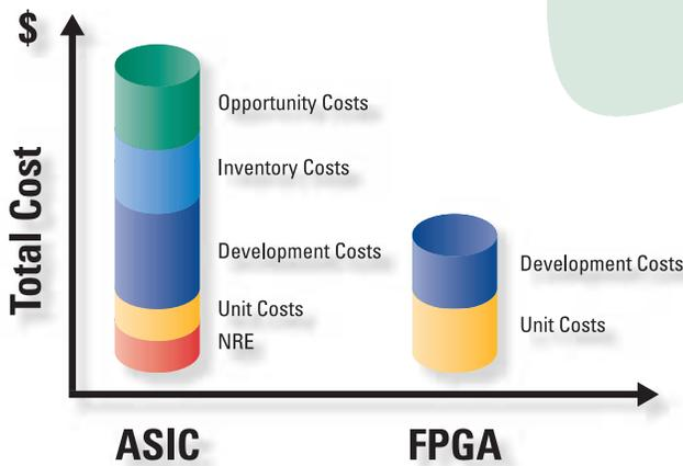
Figure 1 - Cost comparison of ASICs and FPGAs
