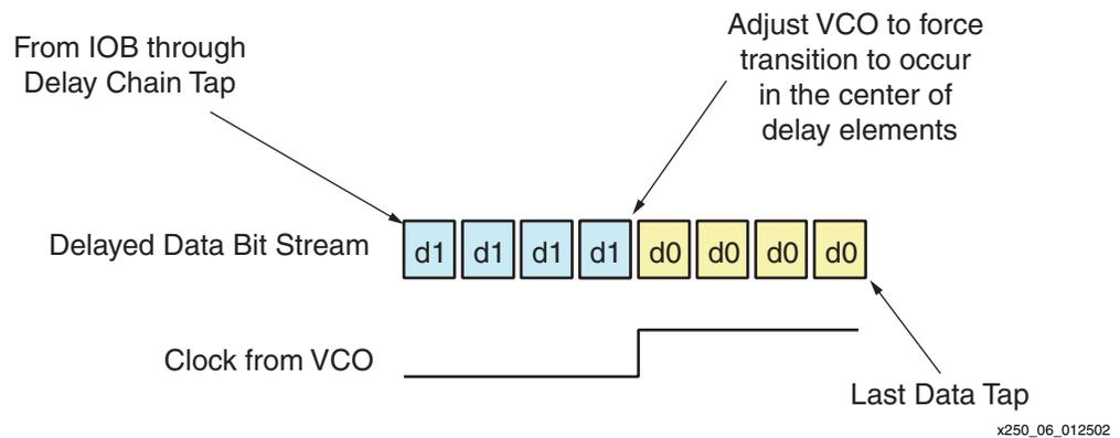
Figure 6: Sampled Delay Line
