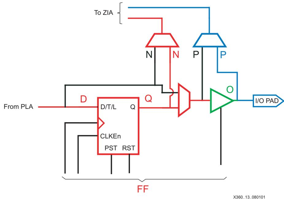
Figure 13: Bi-directional, Registered/Latched Data Path
