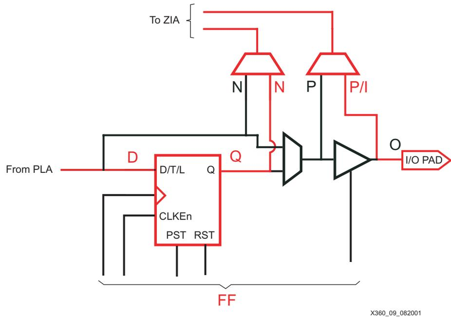
Figure 9: Input with Registered/Latched Node Data Path
