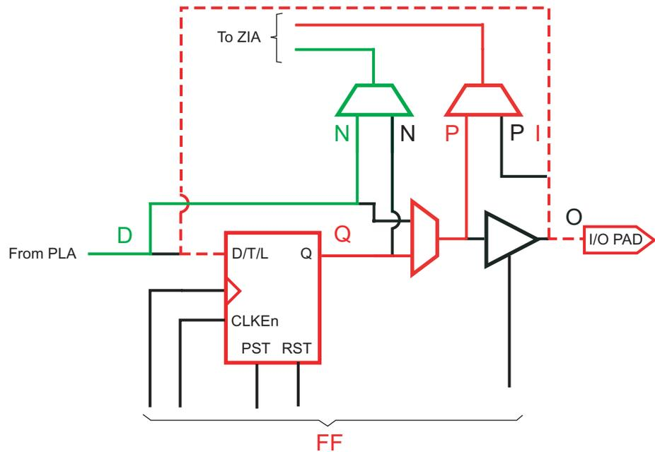
Figure 11: Input Register with Combinatorial Node Data Path
