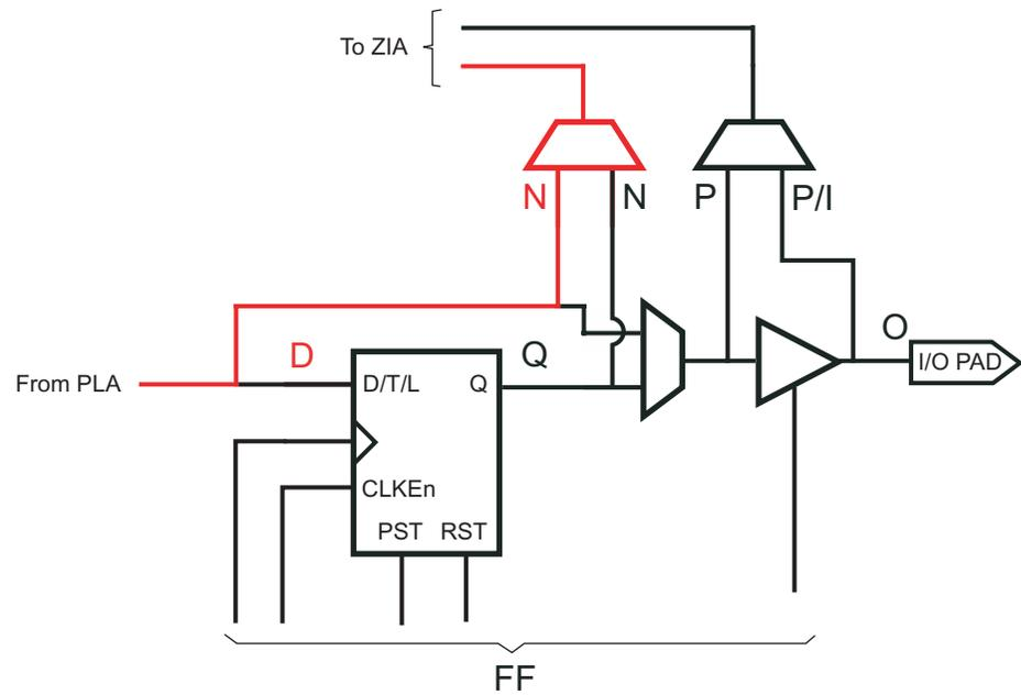
Figure 5: Combinatorial Node Data Path
