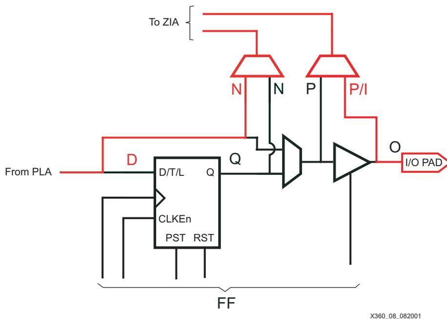
*Figure 8: Input with Combinatorial Node Data Path*
