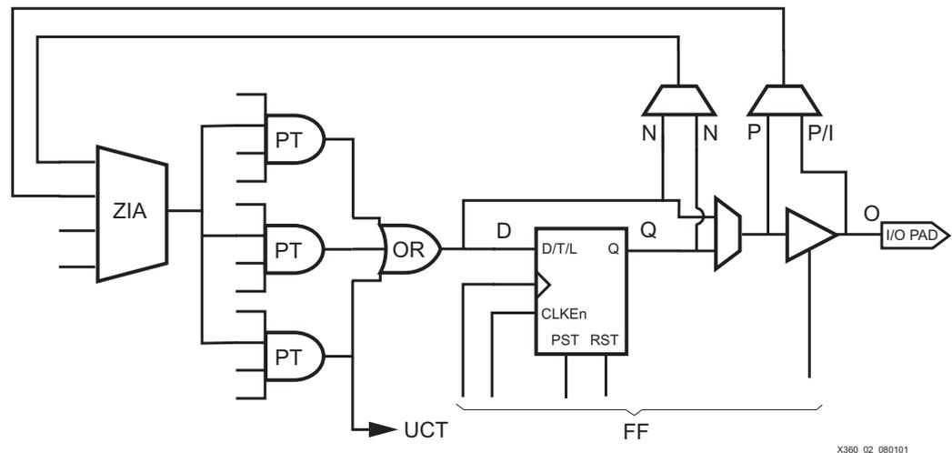
Figure 2: Simplified Power Model for CoolRunner XPLA3 CPLDs
