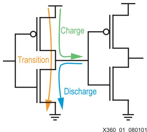
Figure 1: Dynamic Current Through CMOS Inverters
