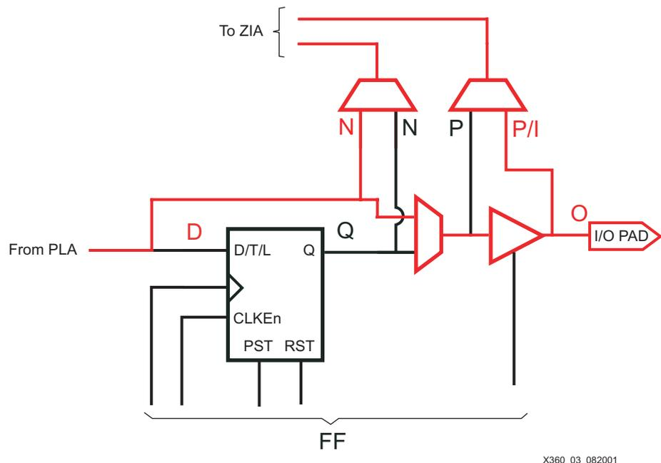
Figure 3: Combinatorial Output Data Path
