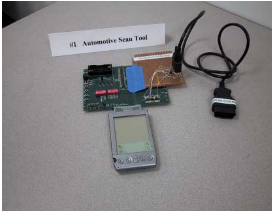
Figure 1: Visor-Based Automotive Scan Tool
