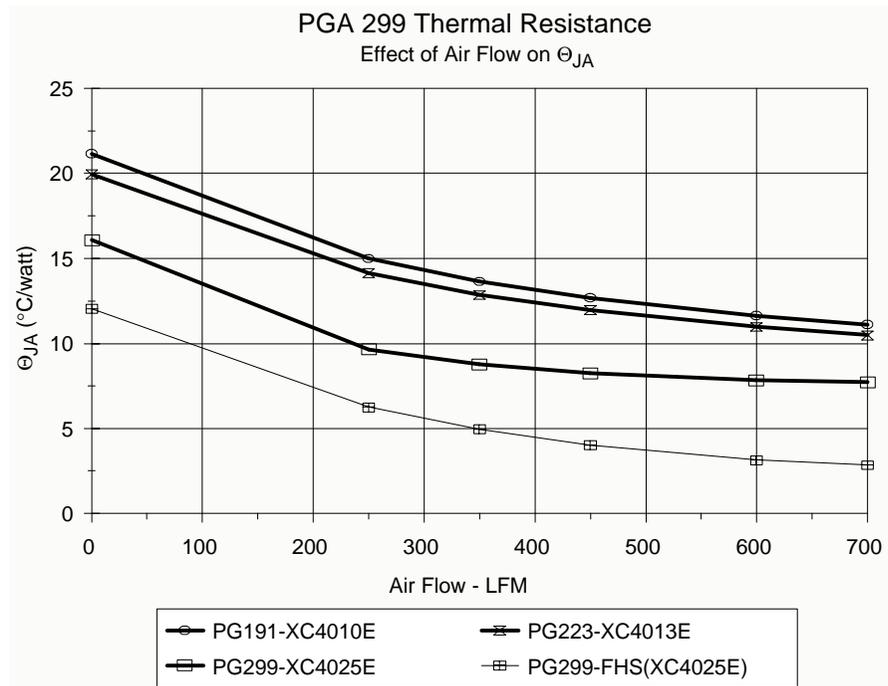
Figure 4: PGA299 Thermal Resistance
