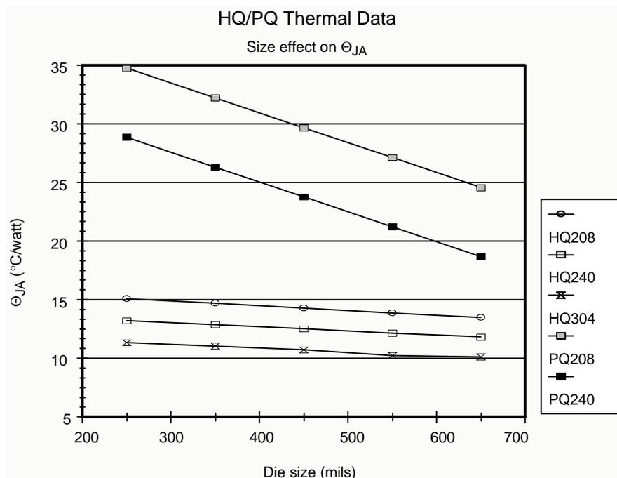
Figure 2: HQ/PQ Thermal Data
