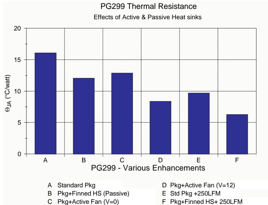
Figure 5: PG299 Thermal Resistance
