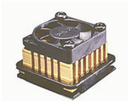
Figure 10: Example of Active Heatsink for BGA (Malico)
