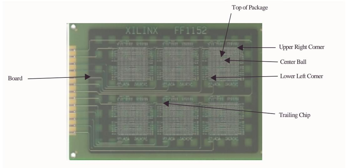
Figure 4: Temperature Measurement Locations
