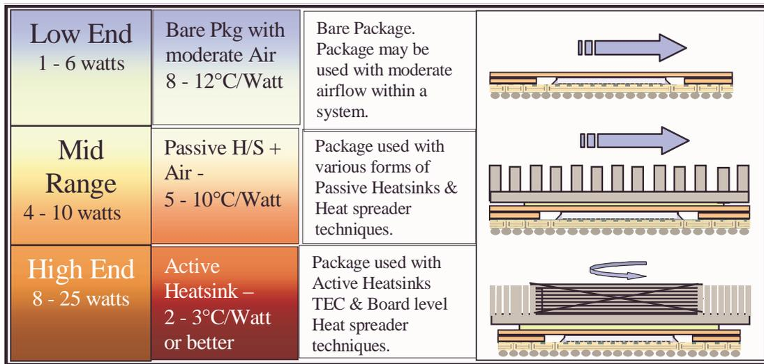
Figure 3: Thermal Management Options for Flip Chip BGA Packages
