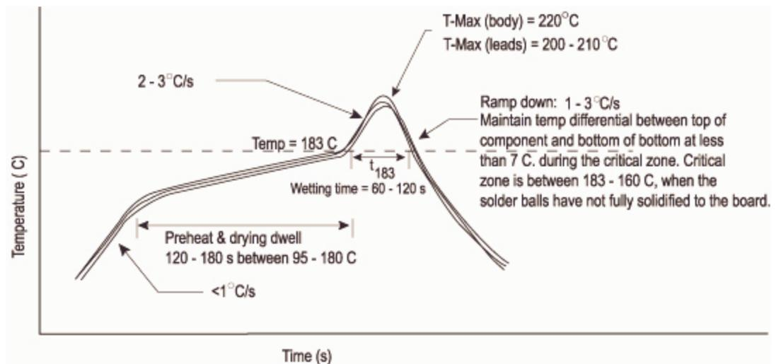
Figure 5: Typical Solder Reflow Profile for BGA
