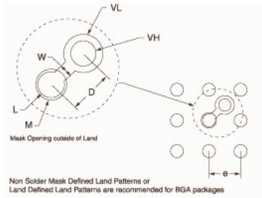
Figure 2: Suggested Board Layout of Soldered Pads for BGA
