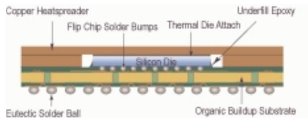
Figure 1: Package Construction
