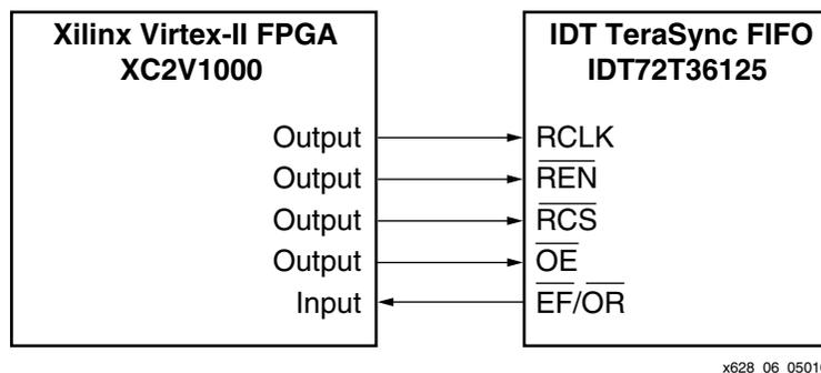
Figure 6: Signals Relevant for Read Operations in IDT Standard Mode
