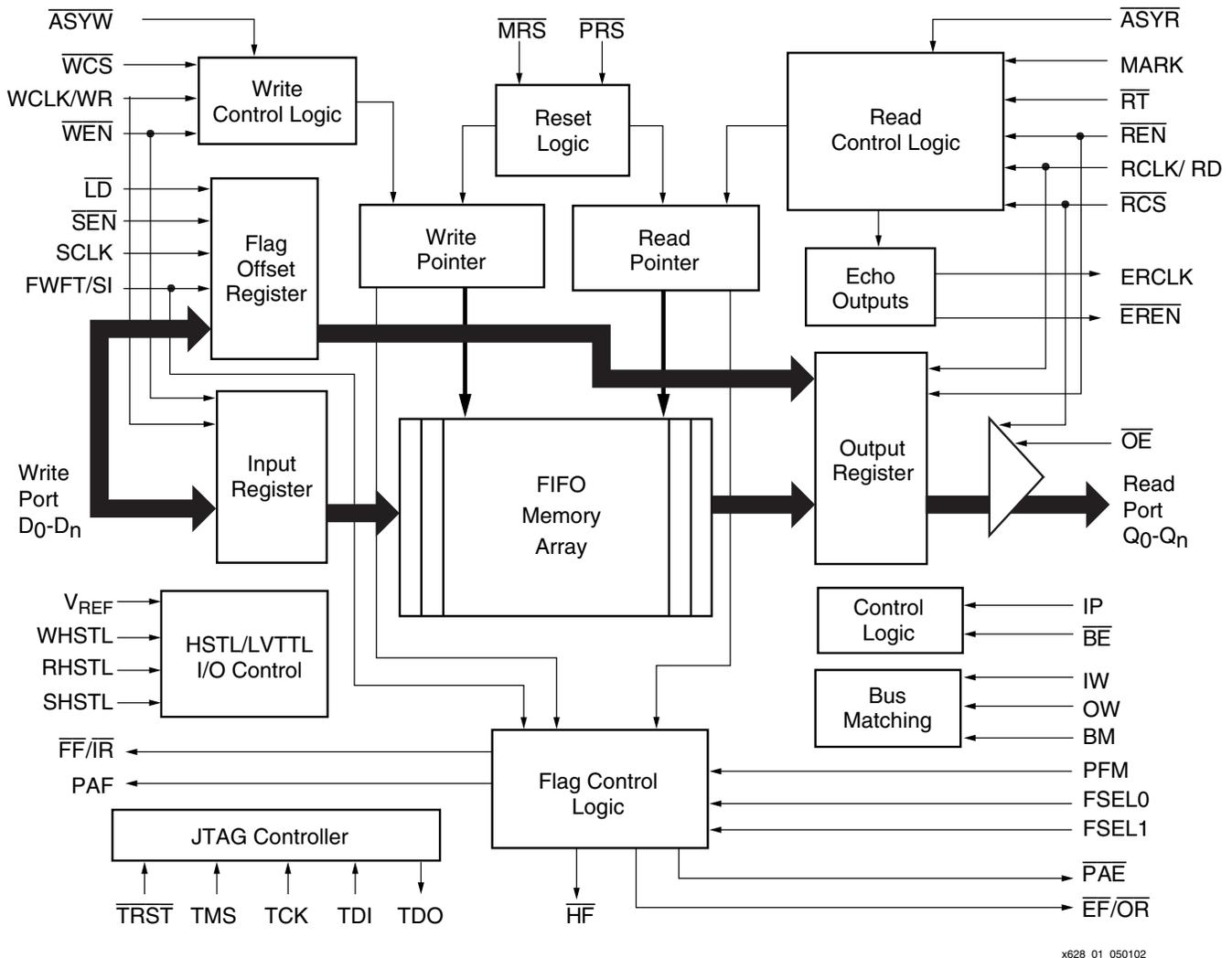
Figure 1: Block Diagram of IDT's TeraSync FIFO
