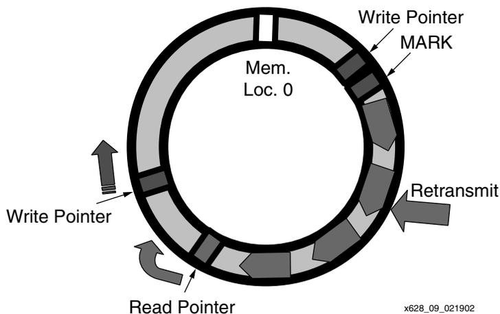
Figure 9: MARK and Retransmit Operation
