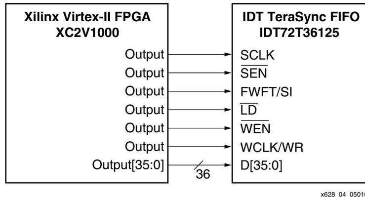
Figure 4: Signals Relevant for Serial and Parallel Programming of PAE and PAF Registers
