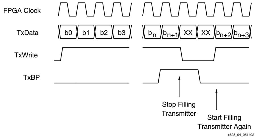
Figure 4: Transmitter Timing
