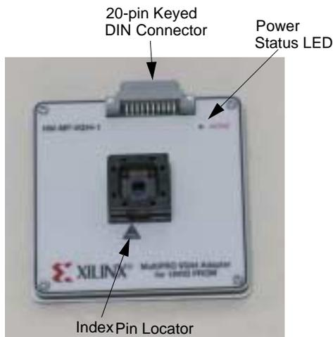
Figure 2: Common Adapter Features
