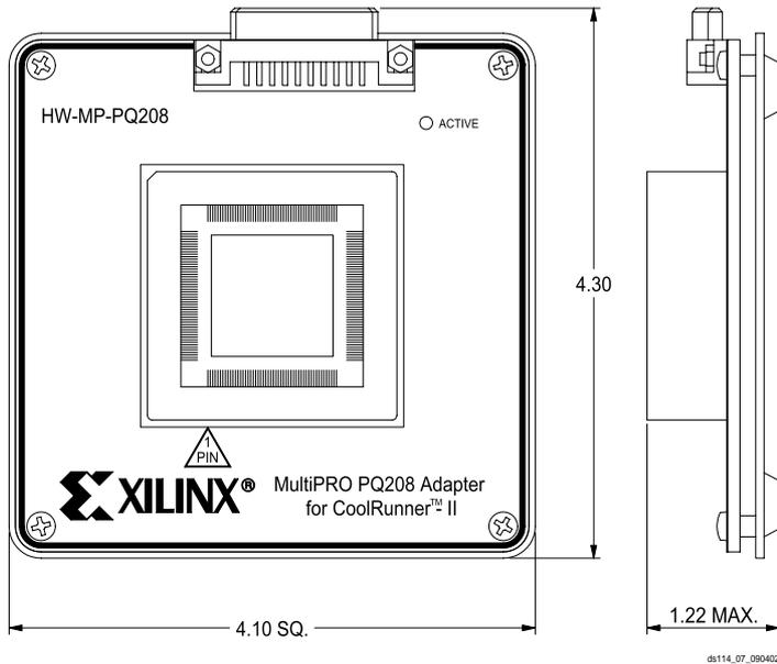
Figure 10: Typical MultiPRO Adapter Dimensions (inches)
