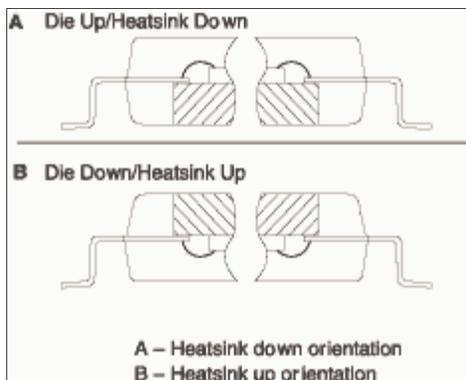
Figure 1: Heatsink Orientation
