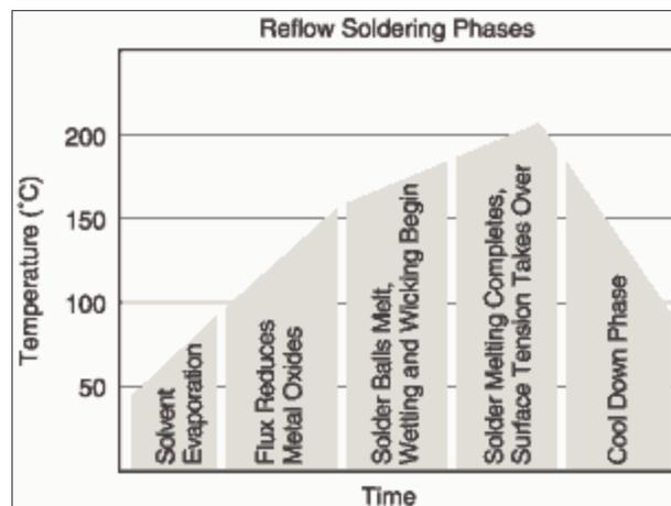
Figure 1: Soldering Sequence
