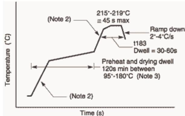
Figure 4: Typical Conditions for Vapor Phase Reflow Soldering
